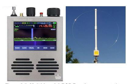
Figure 2.5: **Malahite v1.3 DSP Receiver** connected to <u>K-180WLA</u>—Receive-only **Magnetic Loop antenna** (MLA)
