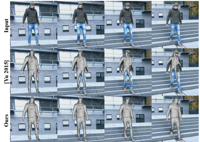
Fig. 13. Qualitative shape comparison between our approach and the template-based monocular non-rigid tracking approach of [Yu et al. 2015]. Our approach is able to reconstruct the motion of the complete sequence, while [Yu et al. 2015] fails after a few frames.
