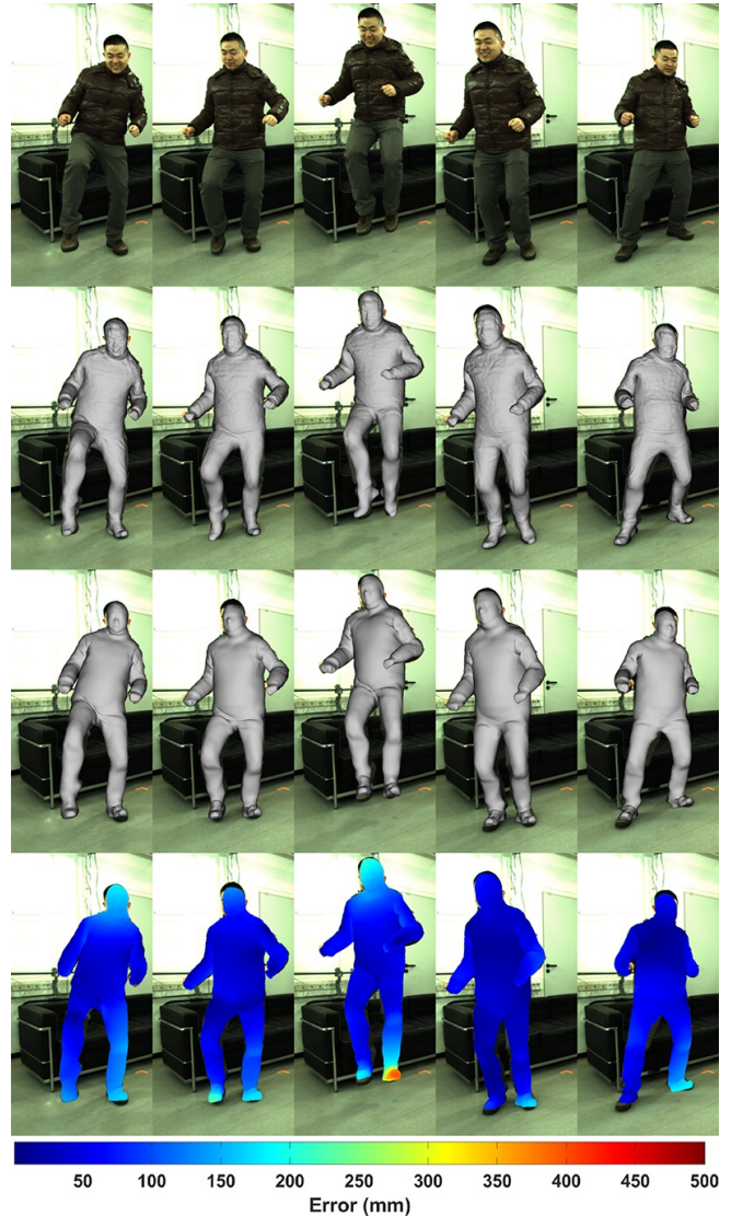
Fig. 18. Qualitative comparison to the binocular stereo performance capture approach of [Wu et al. 2013]. Our monocular approach obtains comparable quality results without requiring explicit depth cues. The per-vertex differences are color coded in the last row. Note, we do not employ full BRDF-based shading-based refinement to obtain smoother results.
