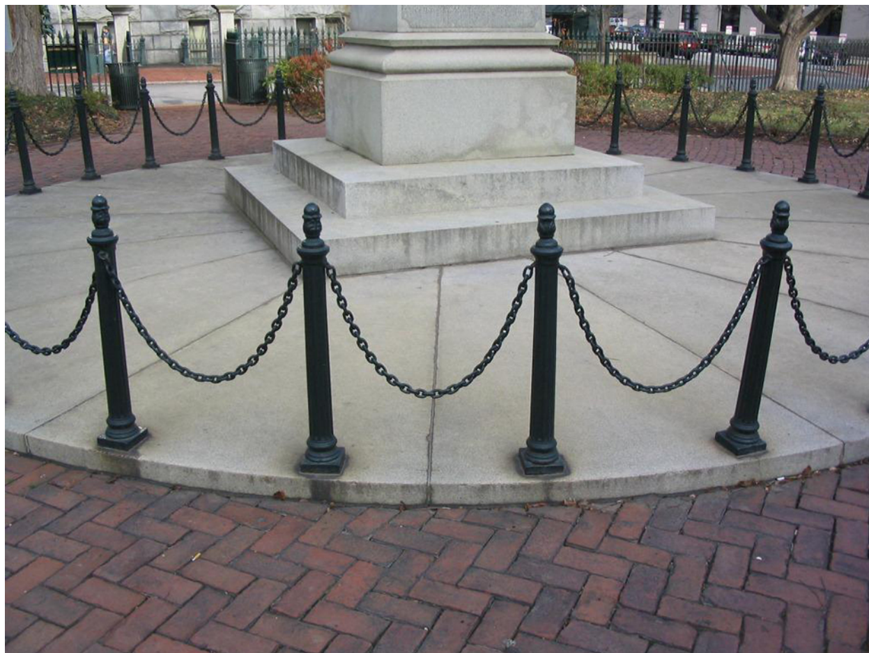
Figure 2.83 Chains between these posts take the shape of a catenary. (credit: modification of work by OKFoundryCompany, Flickr)
