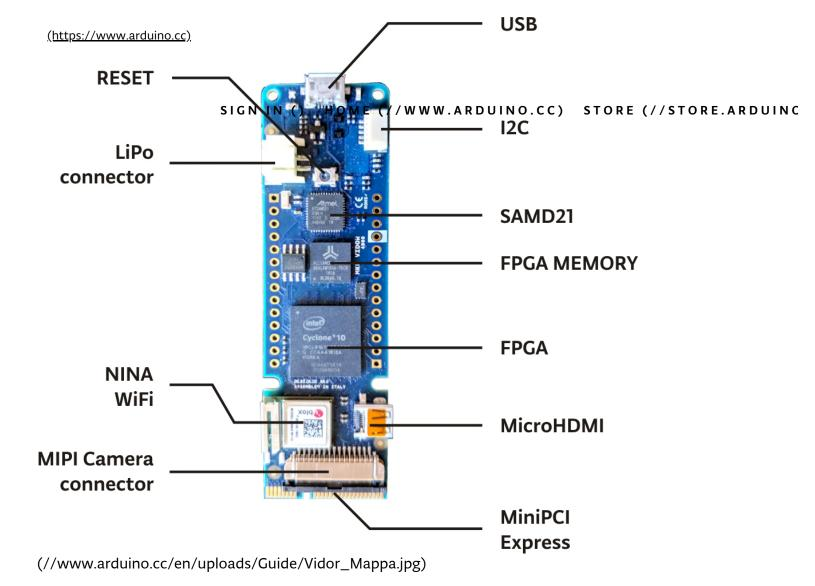
USB - On top of the board you find a standard microUSB port, directly connected to the SAMD microcontroller. This port is seen by the host computer as a Virtual Comm Port and it cn be used to send and receive messages with the usual Serial() function and the Serial Monitor of the Arduino Software (IDE). On the left side of the USB connector you find the BUILTIN\_LED that is red; on the right side a green LED lits
